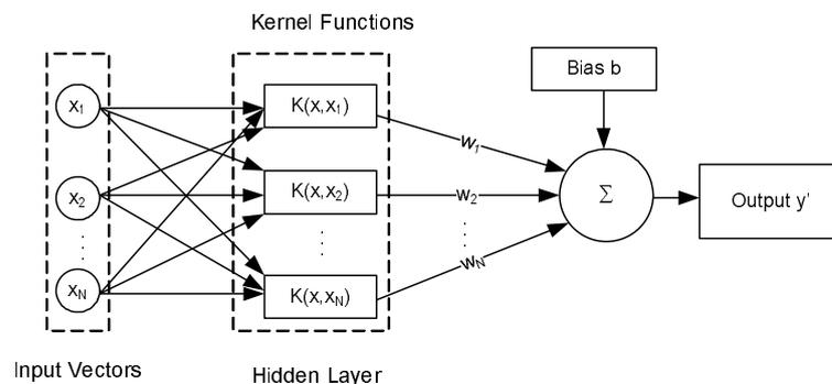
**Fig. 2.** Architecture of the Support Vector Machine. The coefficients  $w$  and  $b$  are the adjustable model parameters.
